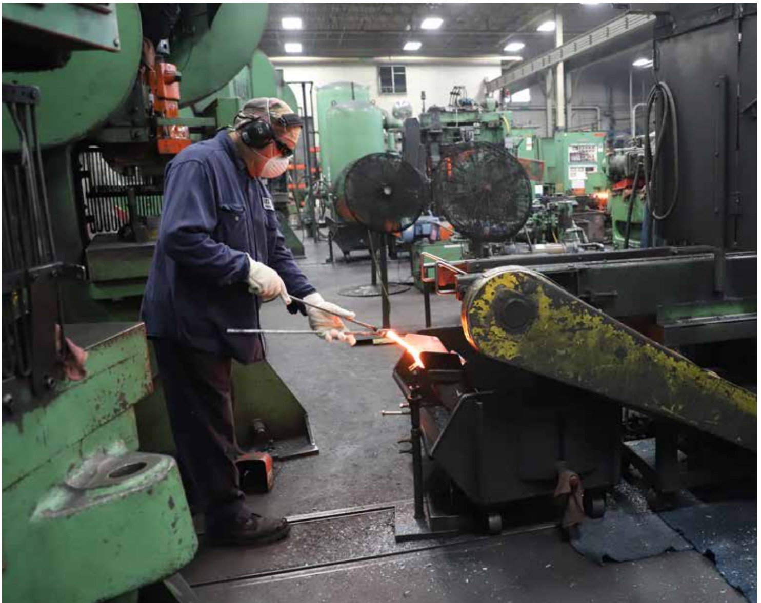
A L-1255 Boilermaker expertly pulls a freshly forged piece fresh from the conveyor.
