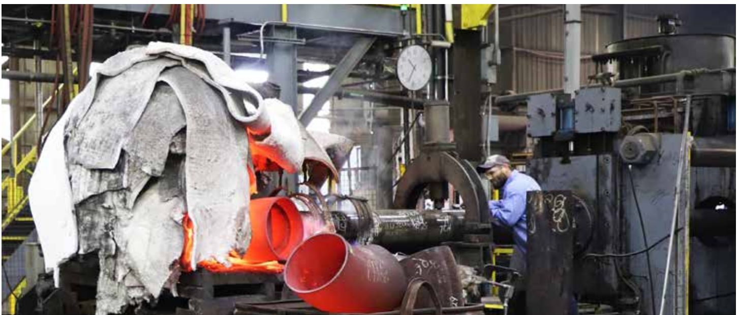
A mandrel maintains the internal shape while a perfect bend forms on a heated fitting.
