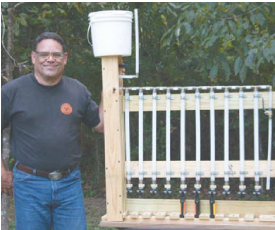
HOLMES DISPLAYS the bottling machine he constructed for his deer scents.
