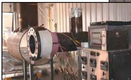
A FIELD HEAT TREATMENT and stress relieving station at the new QCCC training centre in Edmonton.
