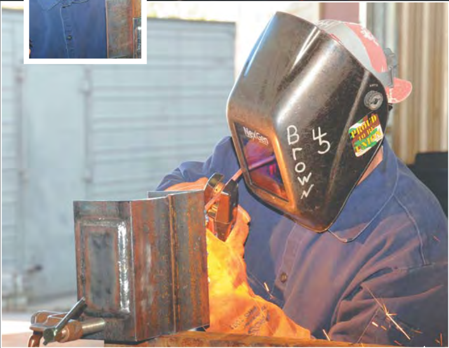
Jason Brown finishes the arc gouging exercise.
