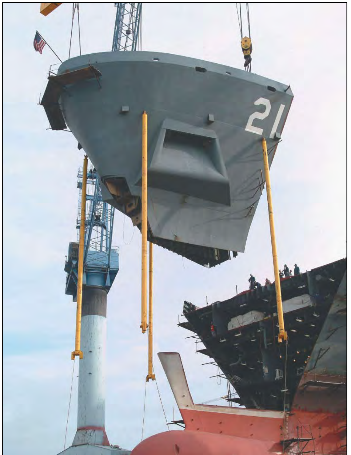
Workers lift the ship's forepeak into position above the bow stem, the vertical, wedge-shaped piece at bottom center of photo. The bow stem is made from salvaged World Trade Center steel. Courtesy of Northrop Grumman Shipbuilding
