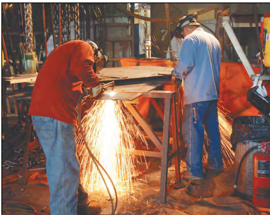
Boilermakers fabricate material to install the VenteX ® system for exhaust ventilation inside a boiler.
