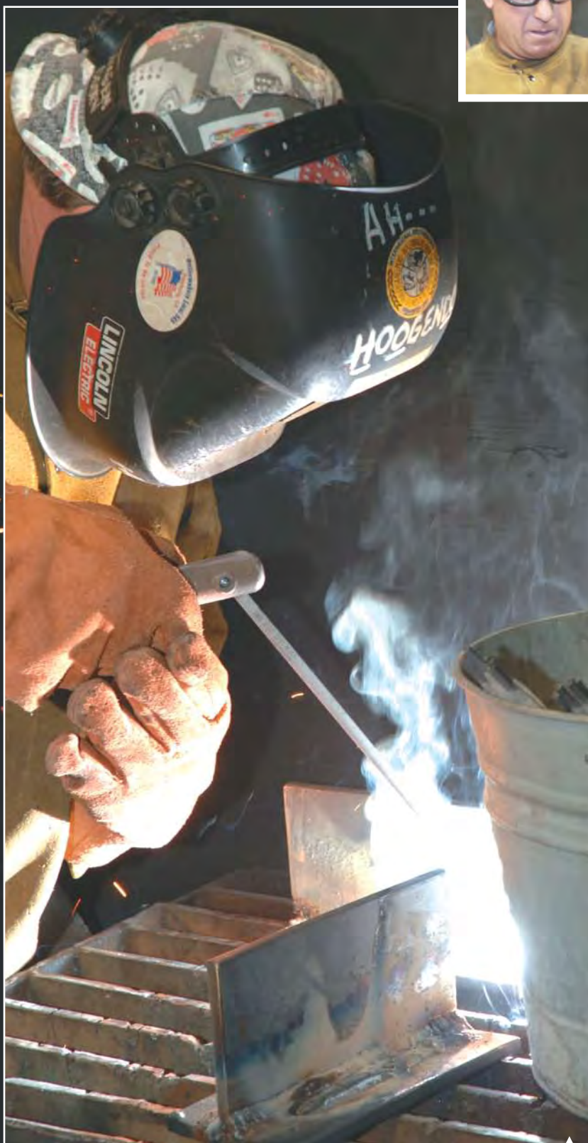
David Hoogendoorn, Local 549, welds a T-joint in the plate welding test, using a 3/16-diameter electrode.
