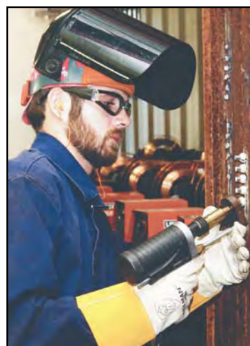
Local 45's Jason Brown works through the stud welding exercise.
