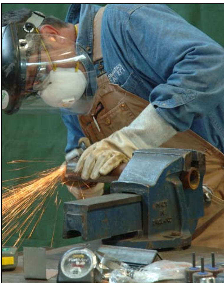
Jean Blanchard, L-271, mills one end of a replacement pup in the waterwall exercise.
