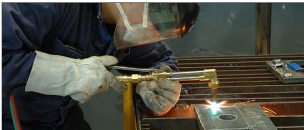
L-146's Geoffrey Moore cuts a lifting lug.
