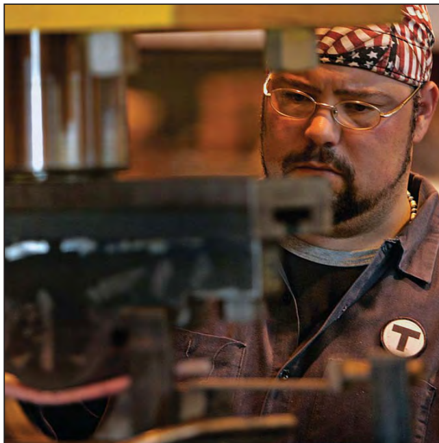
After starting with metal rectangles, Peter Genna, 29, is making pole brackets on a machine in the Everett blacksmith shop. The part is unique to Blue Line trains.
