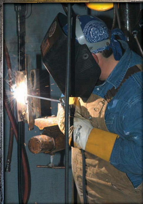
Aaron Pfliger, Local 647, performs a vertical fillet weld.
