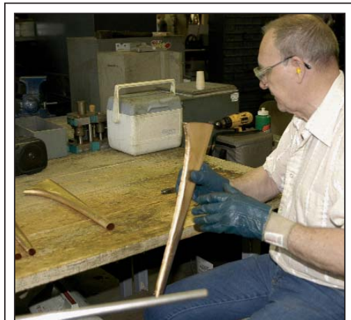
Zelbert Williams forms a trombone bell from a flat piece of brass that is bent and notched together for brazing.
