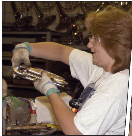
Deb Eldred makes final inspection of a valve section after soldering it together.
