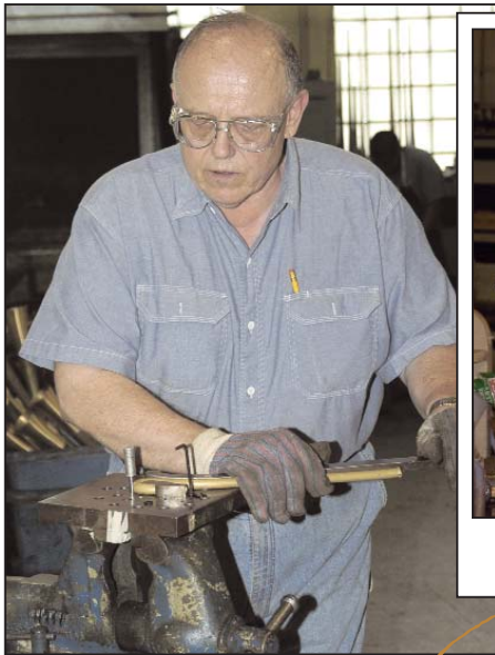
Frank Drohner bends tubes filled with pitch into parts of a slide.
