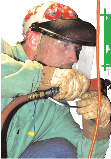
Above: Carl Postlethwait, Local 667, Charleston, W. Va., prepares a panel for insertion of a Dutchman during the welding/bourning portion of the competition.
