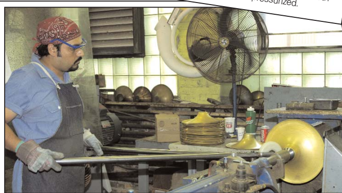
Gerardo Delgado spins a flare against a heavy mold called a mandrel to shape the flare.
