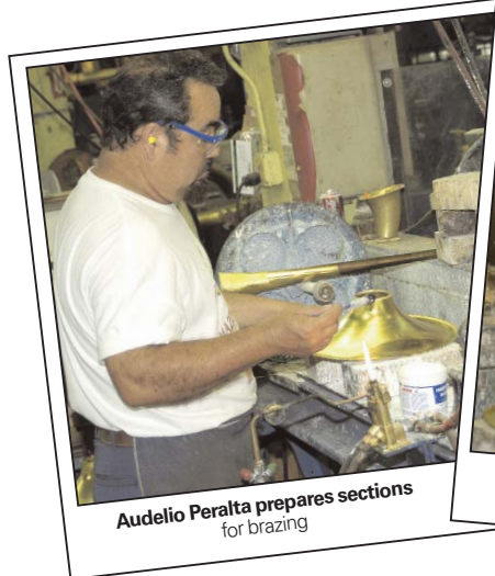
... and then brazes the stem to the flare, creating the French horn's distinctive bell.
