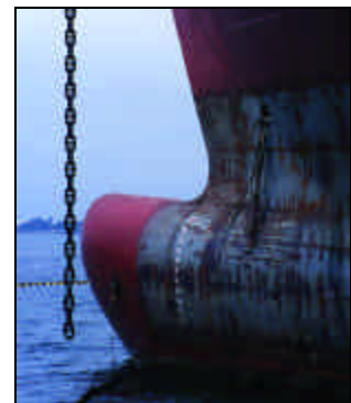
When SWU members built the Midnight Sun (top) they reinforced the bow (above) for icebreaking. Photos by Brian Gauvin
