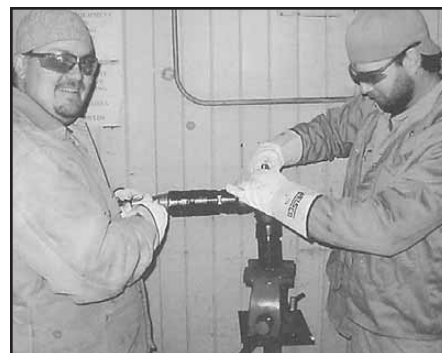
Todd Harris (l.) and Greg Cruise use a milling tube for coupon preparation.
