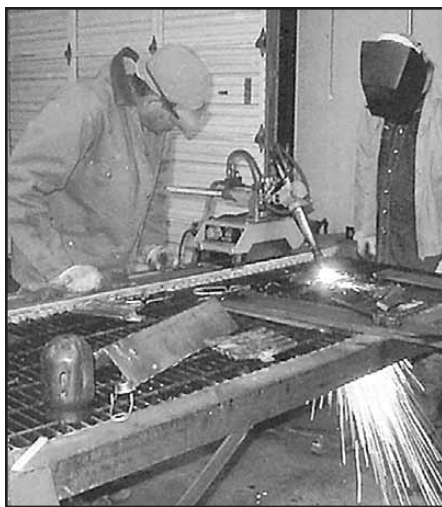
Two apprentices use a trac torch to cut bevels on a plate for weld coupons.
