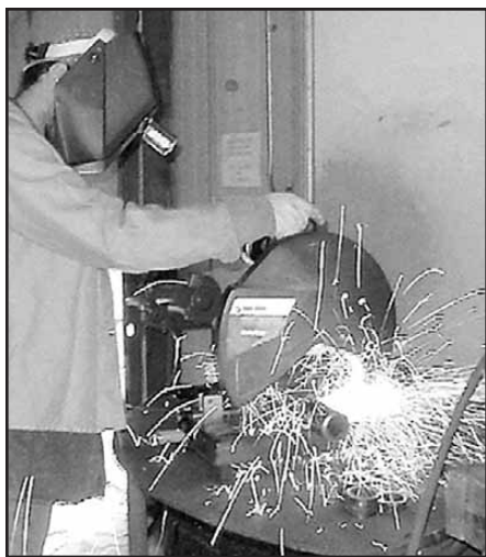
An apprentice uses a cutoff saw to help him get a closer look at a root pass.
