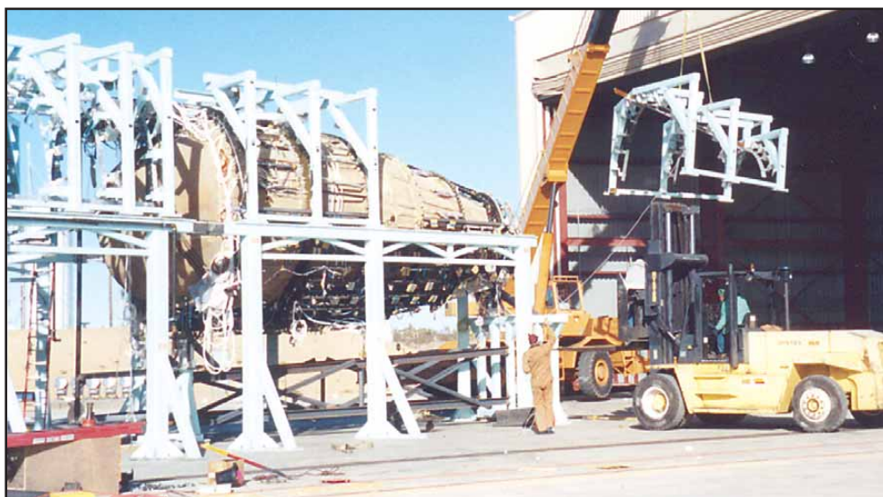
AFTER MOVING THE X-33 to the Edwards Air Force Base, the crew replaces the last piece of the space vehicle's work stand.
