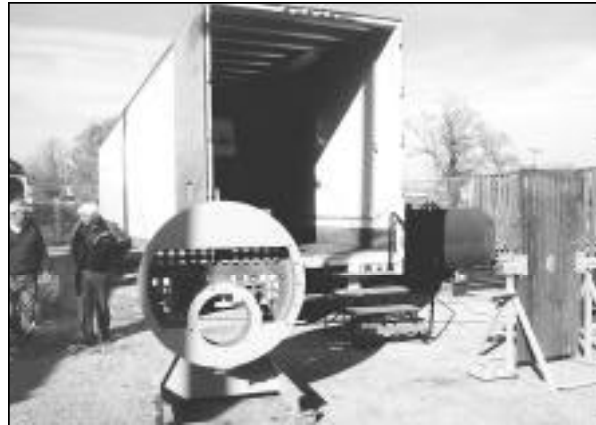
The half-boiler and tube panel pictured above will be securely mounted inside this 42-foot training trailer before transportation to Local 4, where members of the Page, Ariz., local will use this equipment to improve their welding, burning, and tube-rolling skills.
