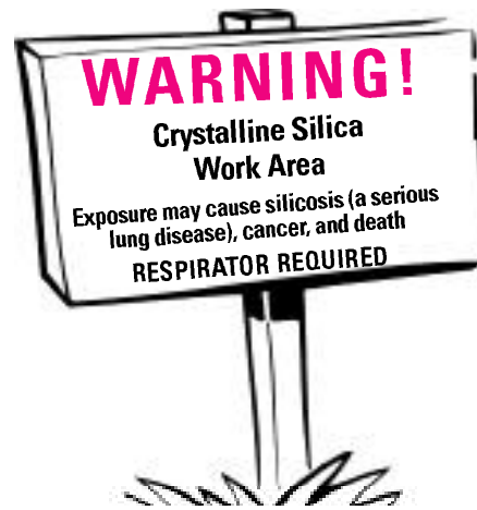
Sample warning sign for silica work area requiring respirators.
