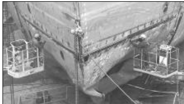
L-680 members are replacing the hulls of three ships for Canada Steamship Lines.
