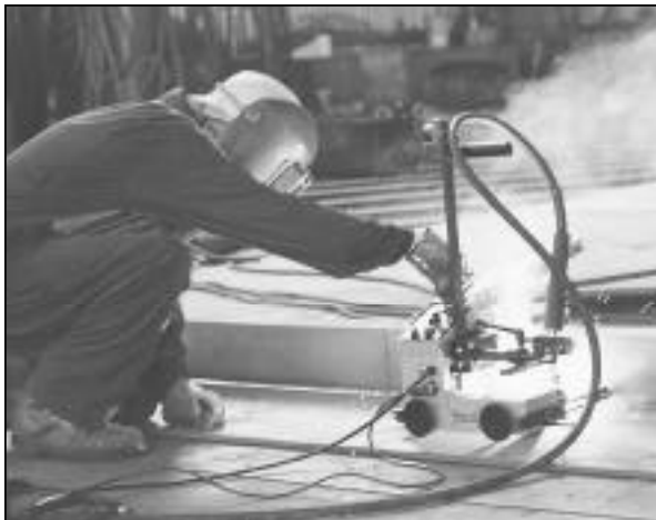
Part of the hull replacement process involves the use of an automatic welder.
