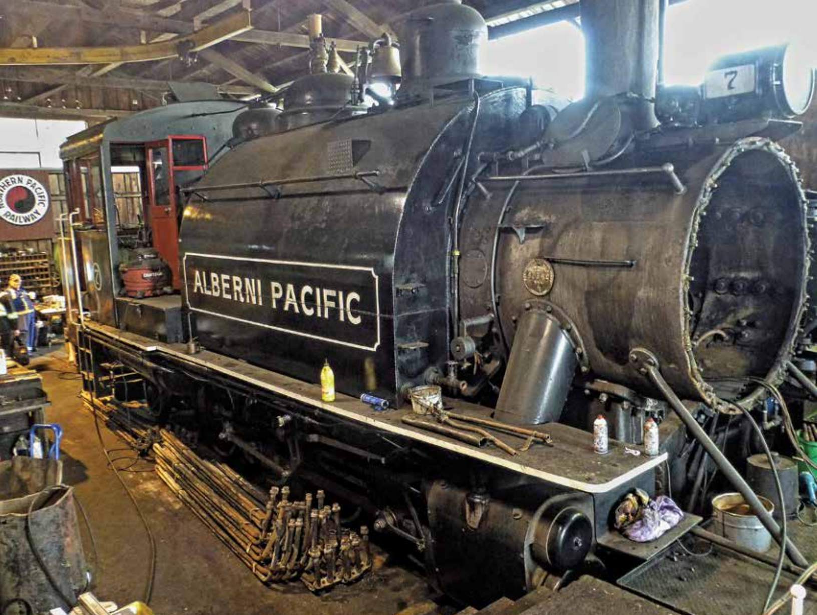
Retired and active members of L-359 strip the 1929 Baldwin Locomotive engine for repair, with its superheaters on the floor waiting to be reinstalled. Photos courtesy of David Hooper, Western Vancouver Island Heritage Society
