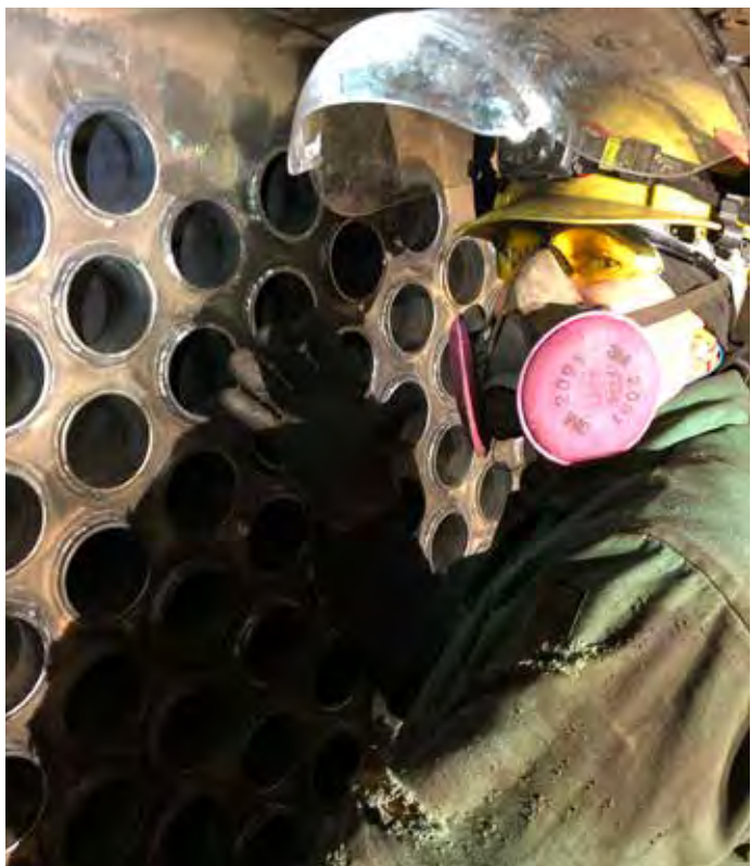
L-34's Don Crerar welds a tube sheet on the Big Boy.
