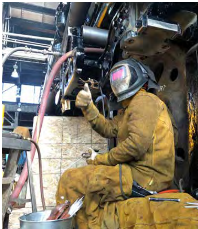
L-34's James Thompson works welding up tapered fit bolts on 4014's frame.
