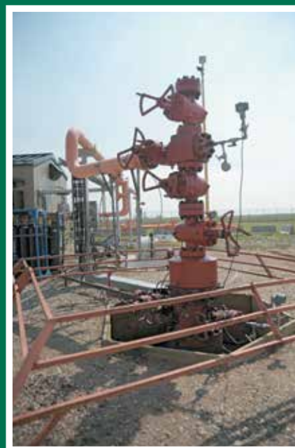
More than three kilometers away from the power station, the CO 2 is injected 3.4 kilometers underground to be safely and permanently stored in porous rock.
