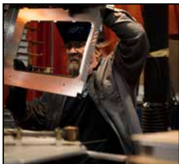
Mark Campbell, fabrication TIG welder, inspects his work after TIG welding a convection oven outer door skin that will hold window glass.
