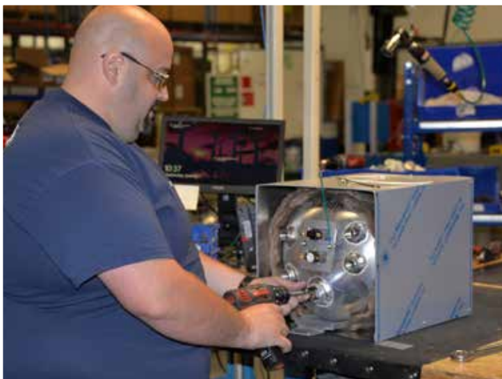
Jeffrey Dukes works on a hot water heater used in yachts and other vessels.
