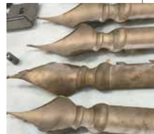
▲ Silicon bronze quill pens before finishing and polishing.
