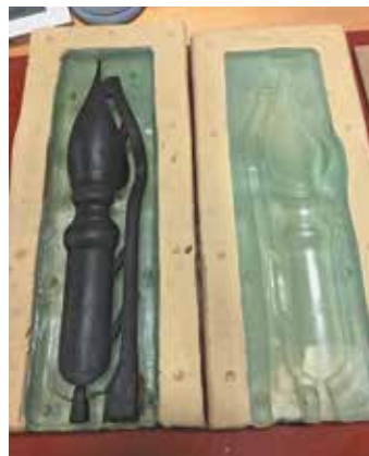
▲ Centuries-old wax casting method, with a rubber mold and casting frame.
