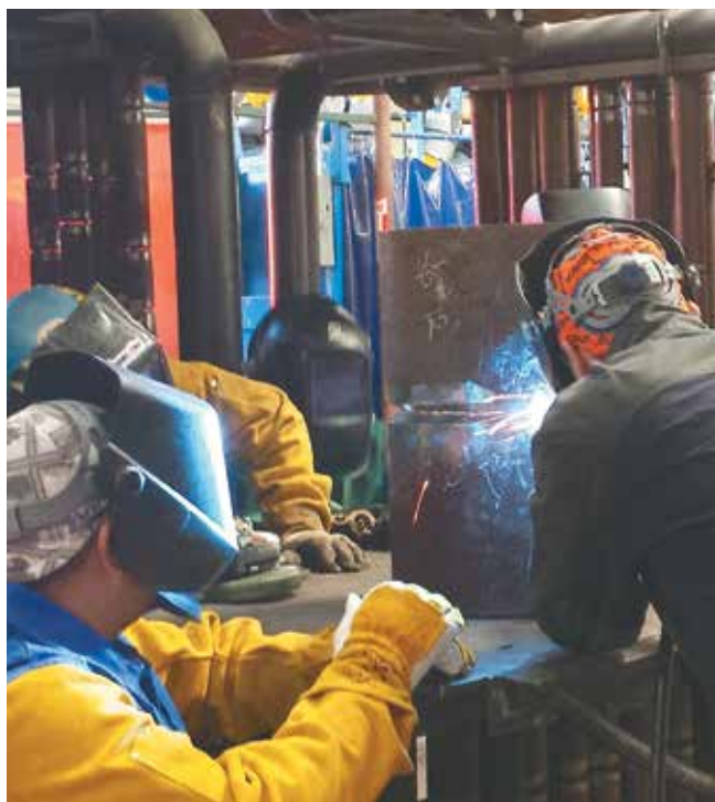
MEMBERS OF L-92 LEARN FLUX-CORE WELDING using Regulated Metal Deposition, which can cut weld times by as much as 50 percent.
